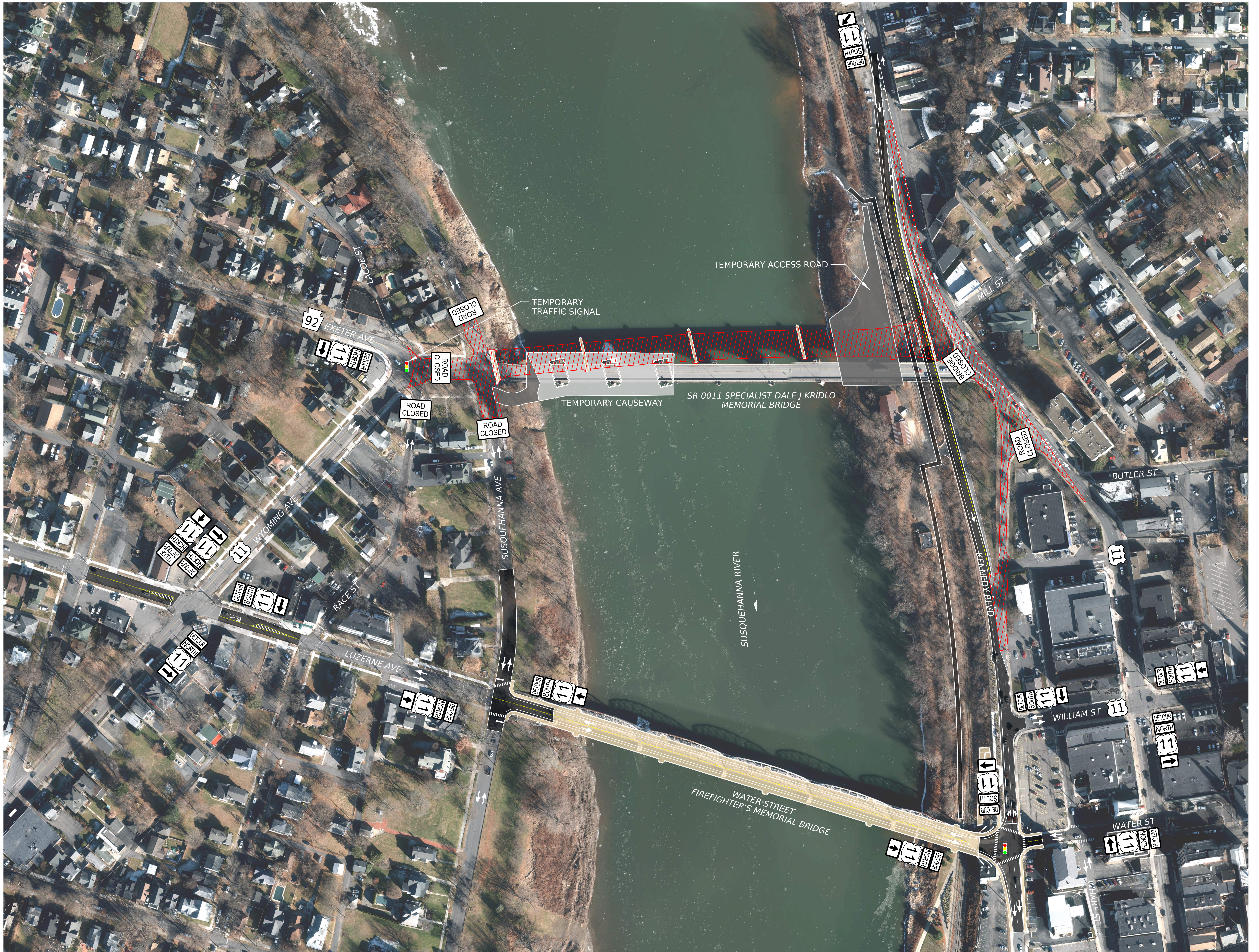
STAGE 4 CONSTRUCTION - TRAFFIC ROUTED TO NEW WATER ST BRIDGE SR11 SECTION 350, LUZERNE COUNTY
