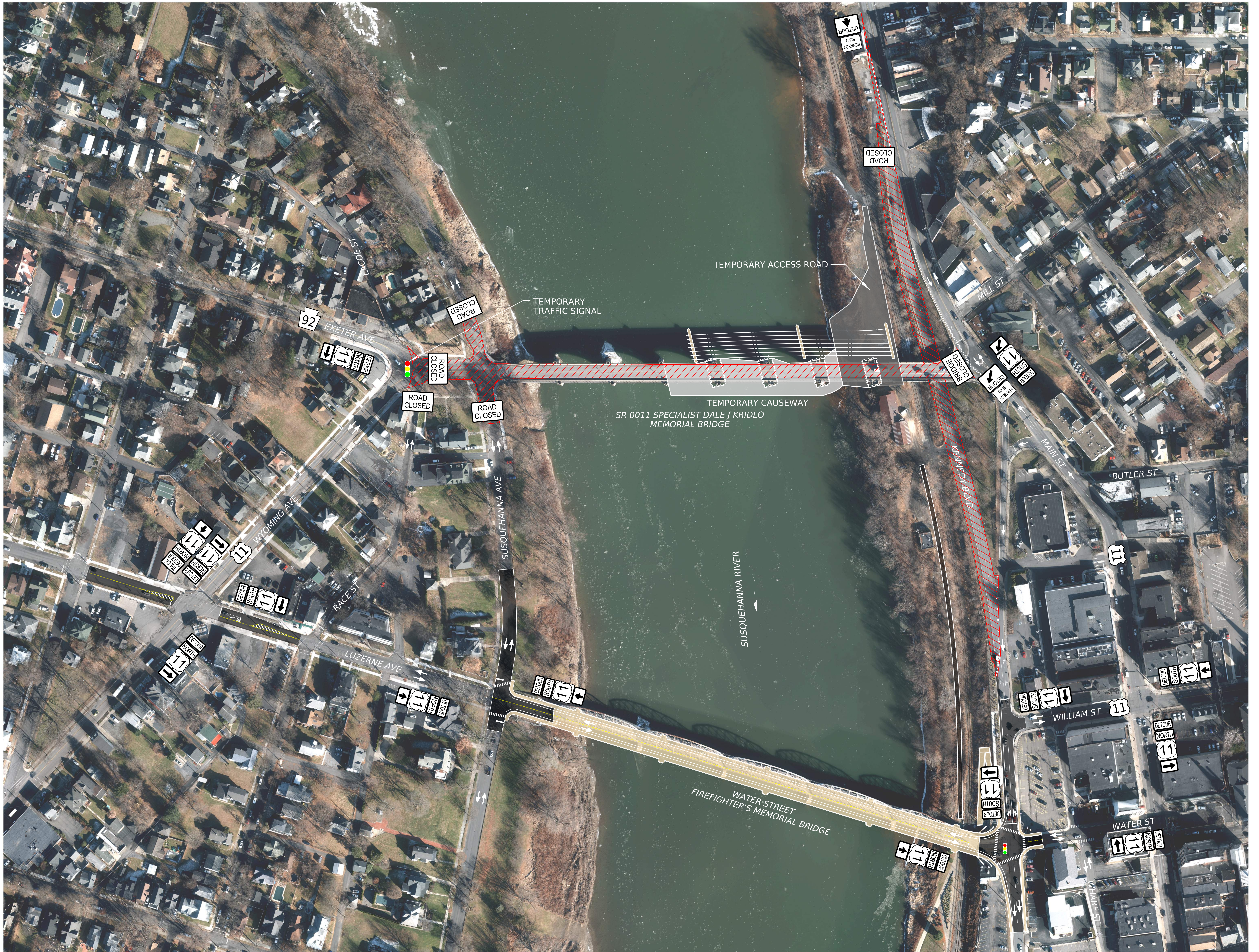
STAGE 3 CONSTRUCTION - TRAFFIC ROUTED TO NEW WATER ST BRIDGE SR11 SECTION 350, LUZERNE COUNTY
