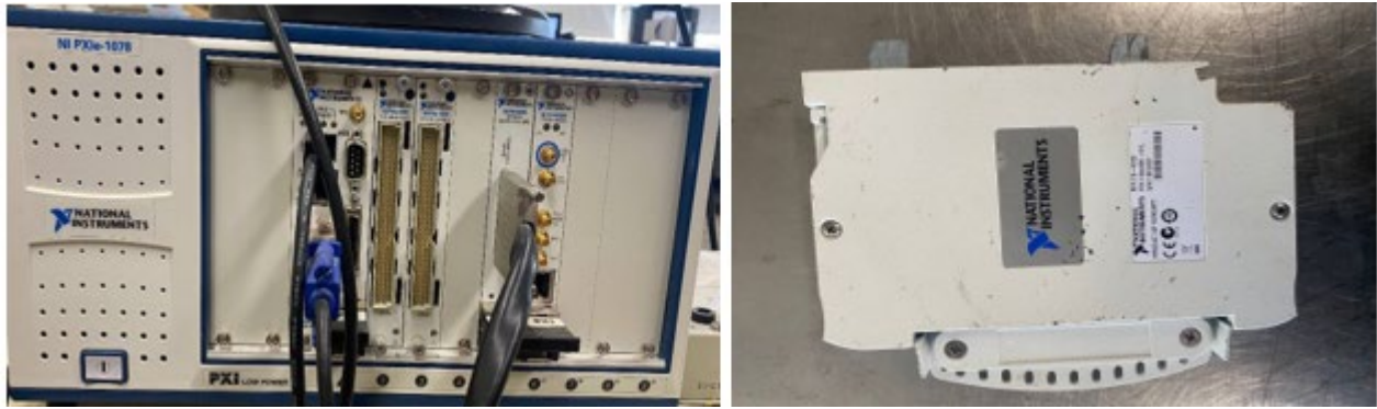
Figure 23. The NI DAQ system (NI PXIe-1078) and Data Acquisition Junction Box (NI TB-4330).
