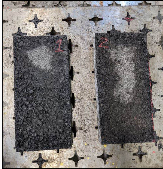
Figure 17. Test slabs cut from larger compacted slab.
