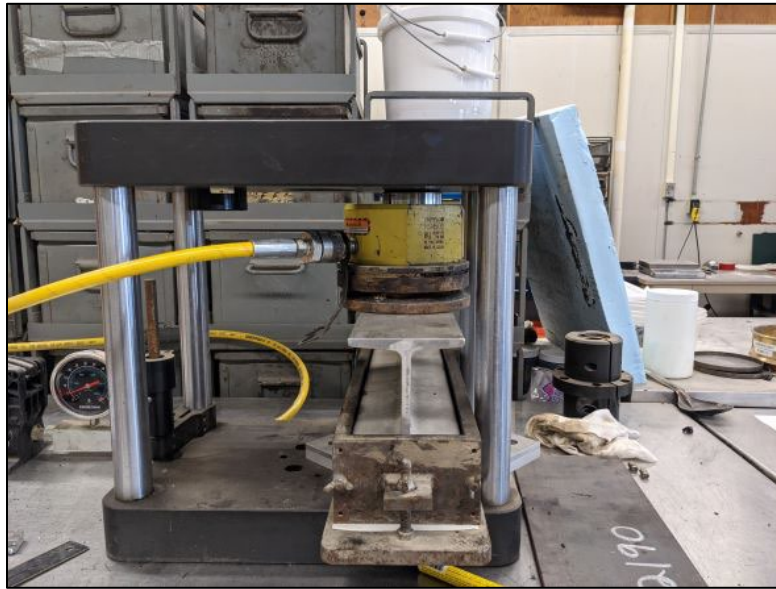
Figure 15. Compaction Mold with ENERPAC and Frame.
