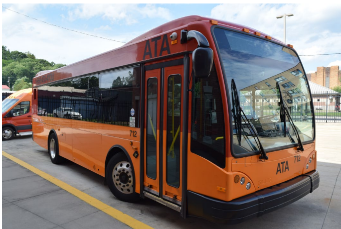
ATA Compressed Natural Gas (CNG) Fixed-Route Bus and Demand-Response Van at the Punxsutawney Bus Terminal
